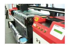
**ZÜND PLOTTER CUTTER** trims to the contour of any shape/size without expensive tooling charges. The intricacy and quantity of cuts required are not limited. Both die cutting from the substrate and kiss cutting are options.
